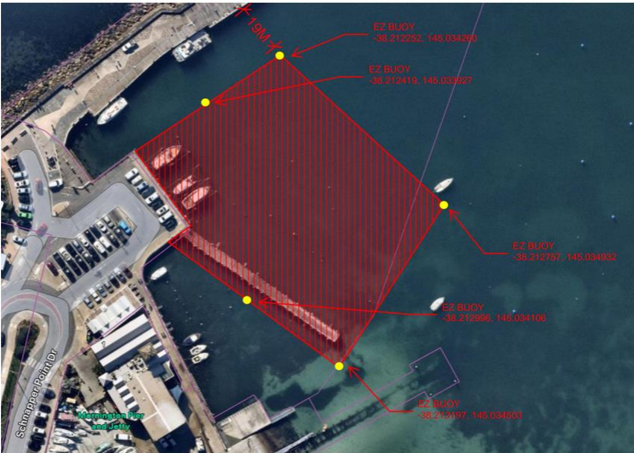
Figure 1 – Fishermans Jetty Demolition Works Exclusion Zone and Buoyage Locations
