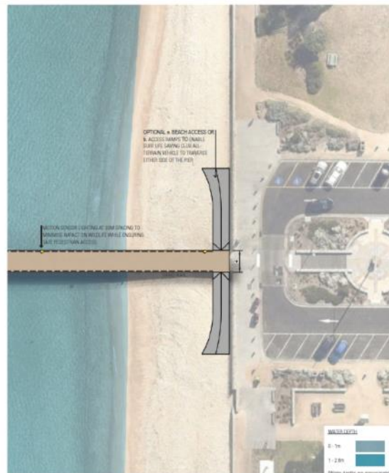
DETAIL PLAN - ABUTMENT 1:200
