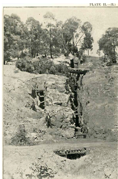
FISSURED CENTRE COUNTRY, WITH LARGE BODY OF QUARTZ, EUREKA LINE OF REEF. Looking south; quartz up to 40 feet wide, centre portion not stoped. Walls diverge in depth, forming east and west legs of a saddle reef.
