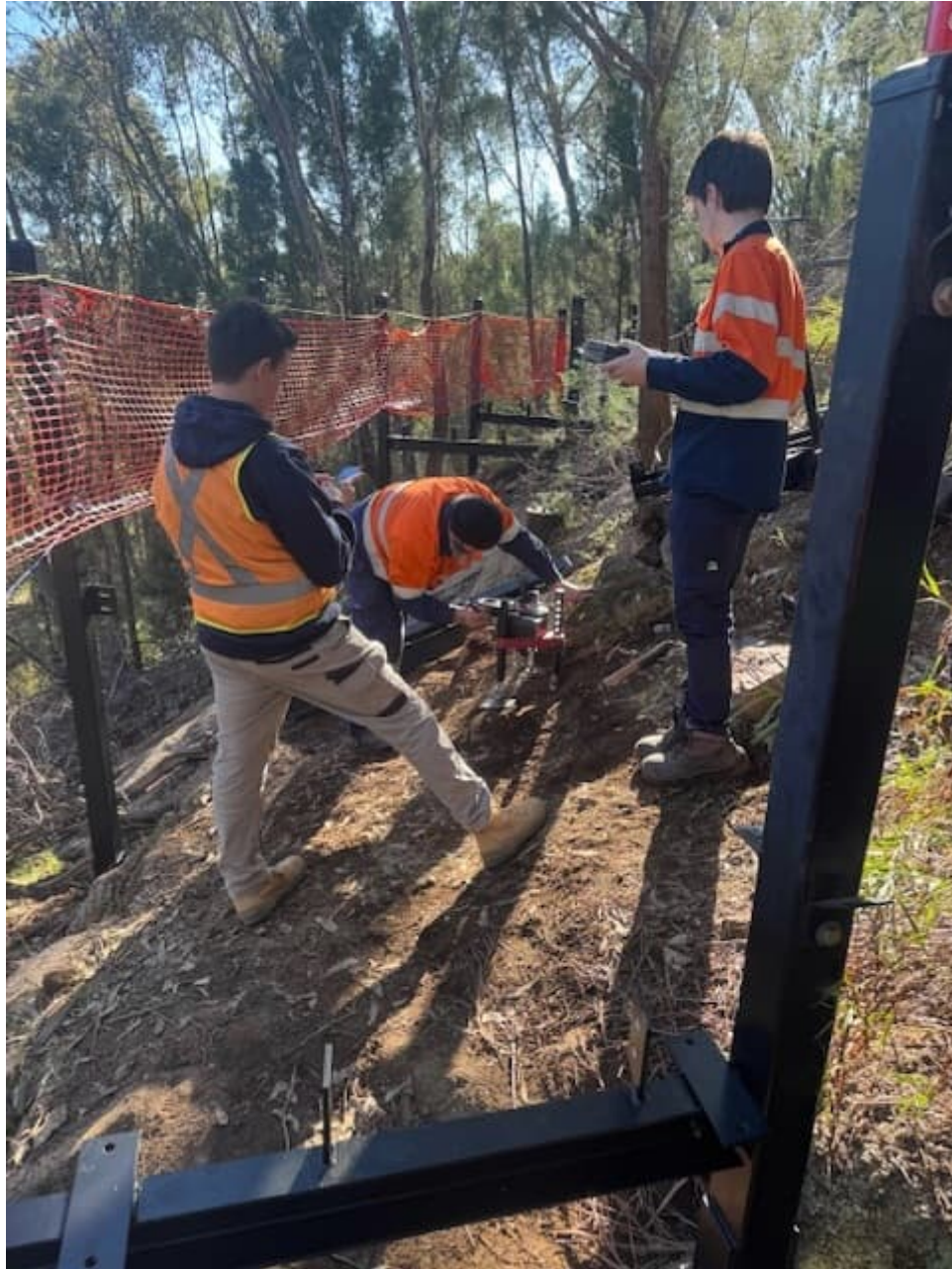
Photo 21 Bolt Testing (all 6 locations passed)
