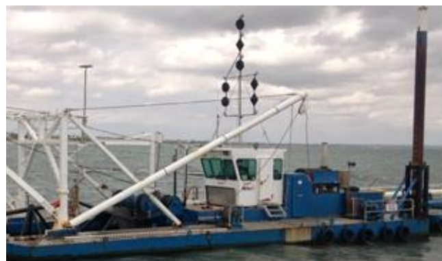
The two diamond shapes on the dredger indicate the safe side for vessels to pass
