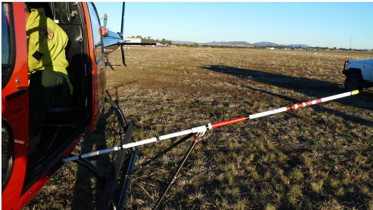
**Fig. 5** Distance boom mounted on the left-hand side of the Eurocopter AS350 Écureuil helicopter used in the 2019 surveys. The distance bins used in the surveys (0-20 m, 20-40 m, 40-70 m, 70-100 m and 100-150 m) are indicated by the black bands on the boom.
