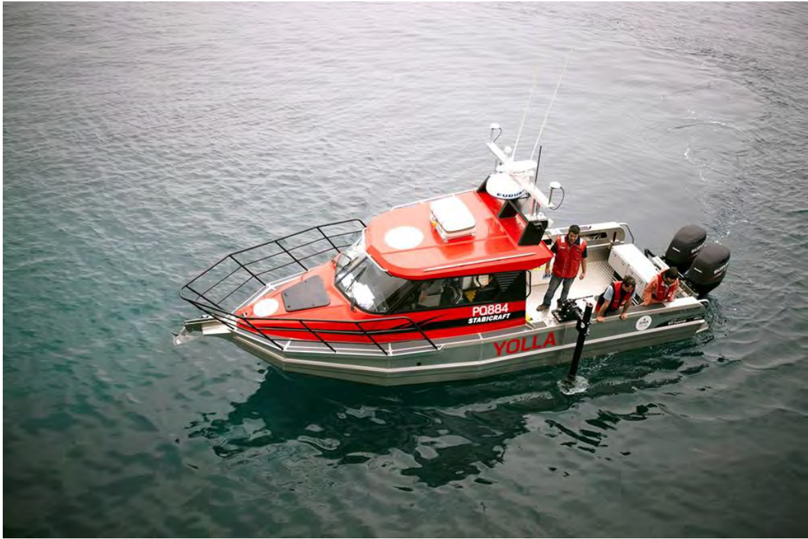
Figure 2 Yolla RV with sonar head mounted on a pole over the portside.
