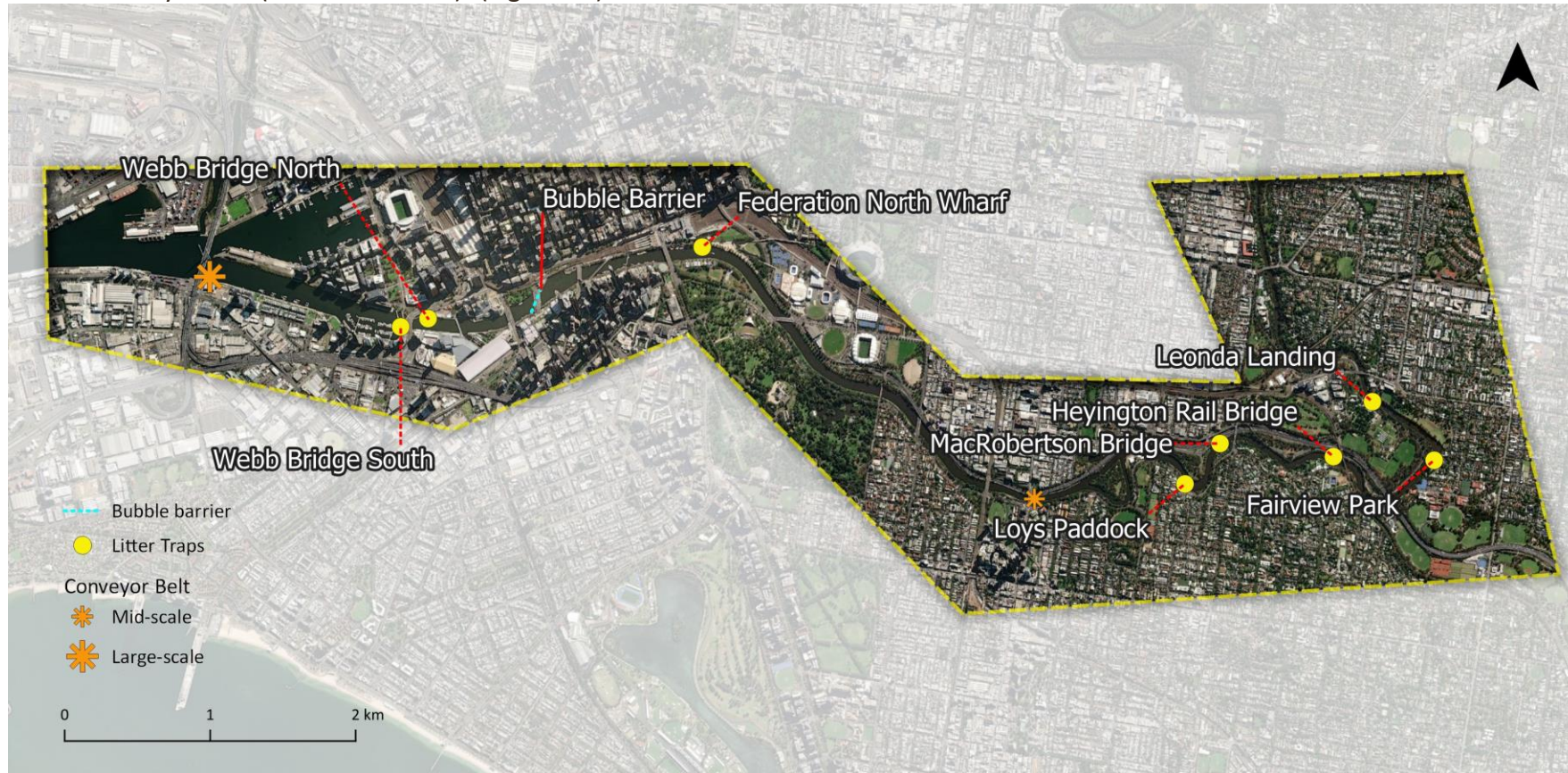
Figure 21. Yarra River - Scenario 3: 8 litter traps and booms, 1 bubble barrier, 1 mid-scale conveyor belt + 1 large scale conveyor belt.
