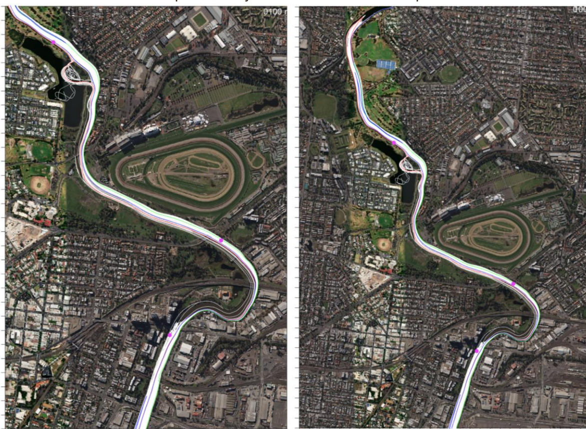
Figure 12. View of the litter trap locations along the Maribyrnong River (pink dots) with the litter tracks of all the particles released (white) along with example individual tracks in blue, green and red.
