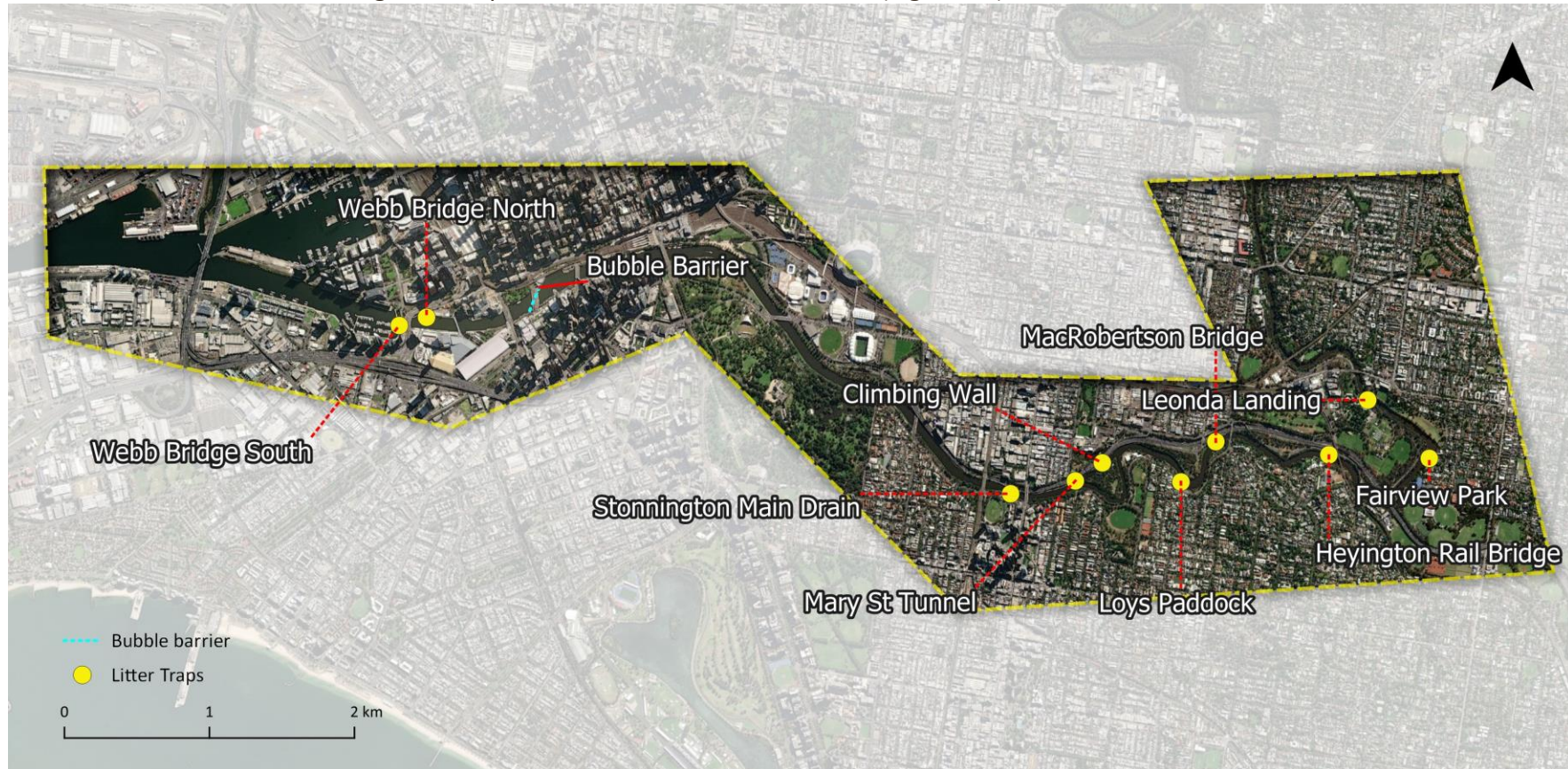
Figure 19. Yarra River - Scenario 1: 10 litter traps and booms, and 1 bubble barrier.
