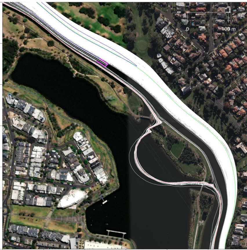
Figure 7. Litter tracks (white) along the Maribyrnong River section near Edgewater Marina under typical flow conditions, with example individual tracks shown in blue, red and green.
