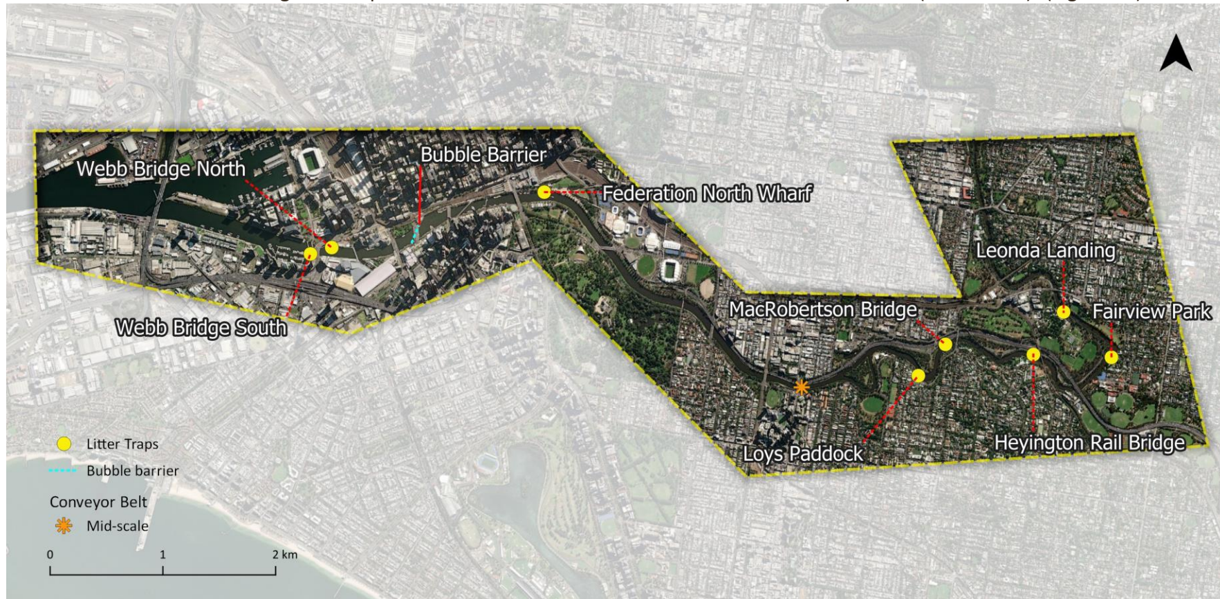
Figure 20. Yarra River - Scenario 2: 8 litter traps and booms, 1 bubble barrier, 1 mid-scale conveyor belt.
