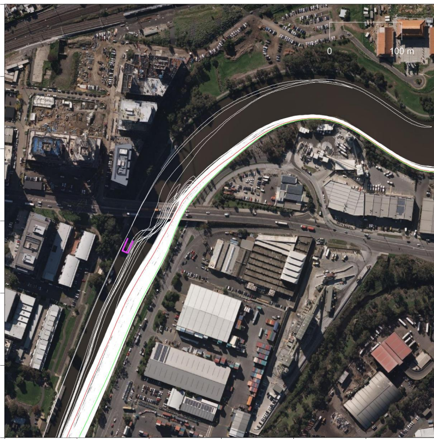
Figure 9. Litter tracks (white) along the Maribyrnong River section near Dynon Bridge under typical flow conditions, with example individual tracks shown in red and green.
