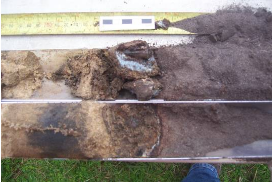
Figure 68 Burnt material and glass identified in a core sample.
