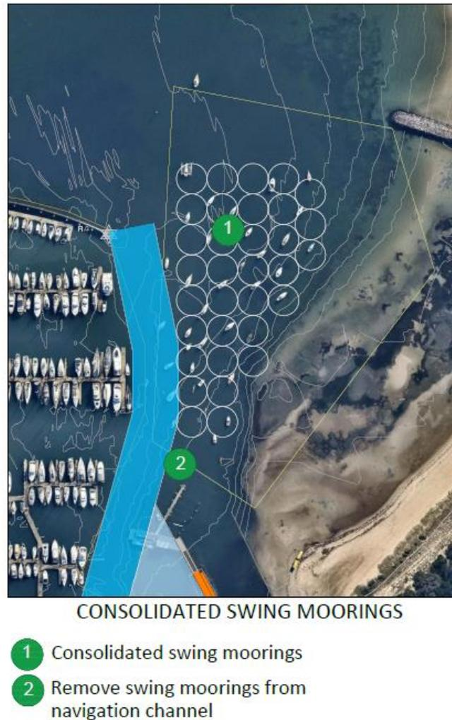
**Figure 10 – Proposed Mooring Ground Arrangement grid (Aerial image: Nearmap 29/10/2021)**
