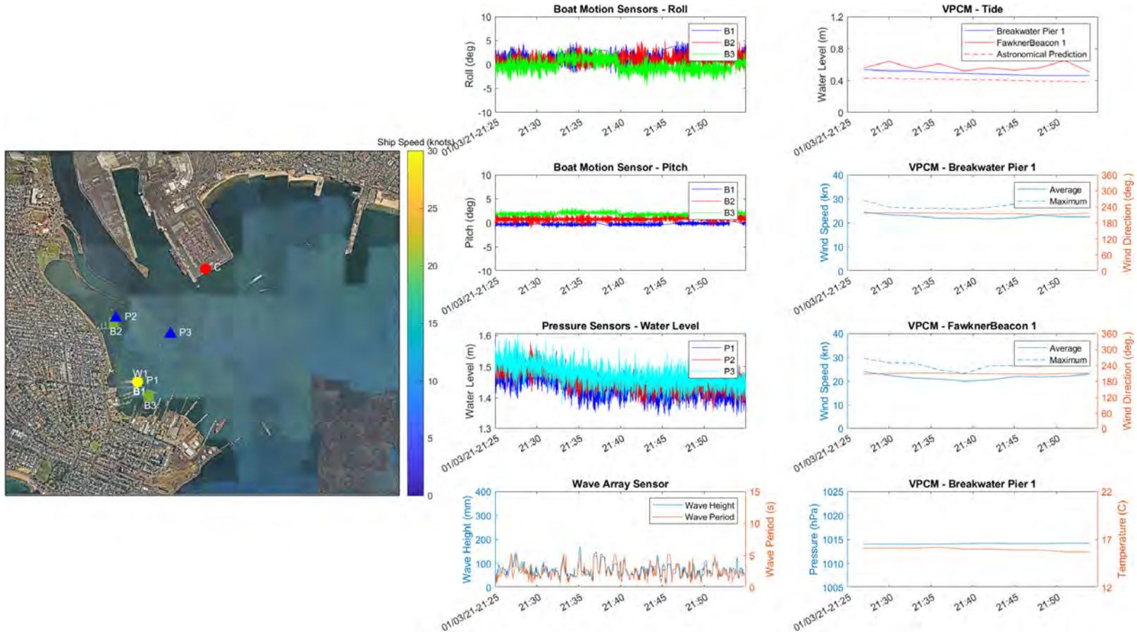
Figure 2.13 Summary diagnostic plot of marine traffic, metocean conditions and moored boat motions on 1 March 2021 from 21:25 to 21:55
