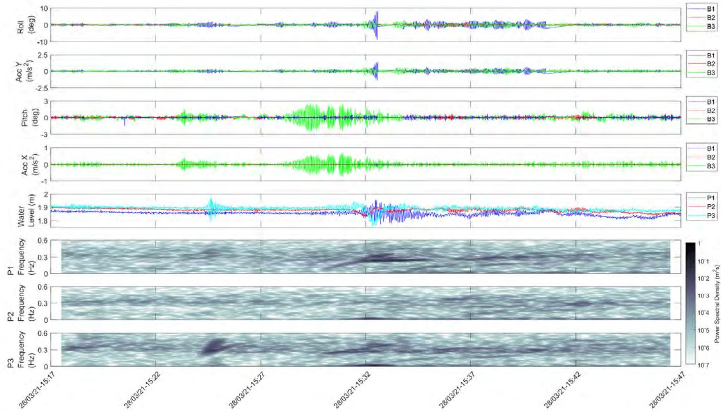
Figure 2.23 Spectrogram and diagnostic plot for an example event detection with a passing Tanker vessel
