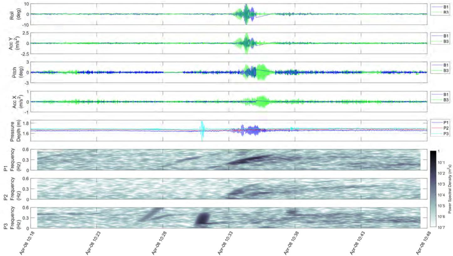
Figure 2.18 Spectrogram plot for metocean conditions and boat motion accelerations on 8 April 2021 from 10:18 to 10:48
