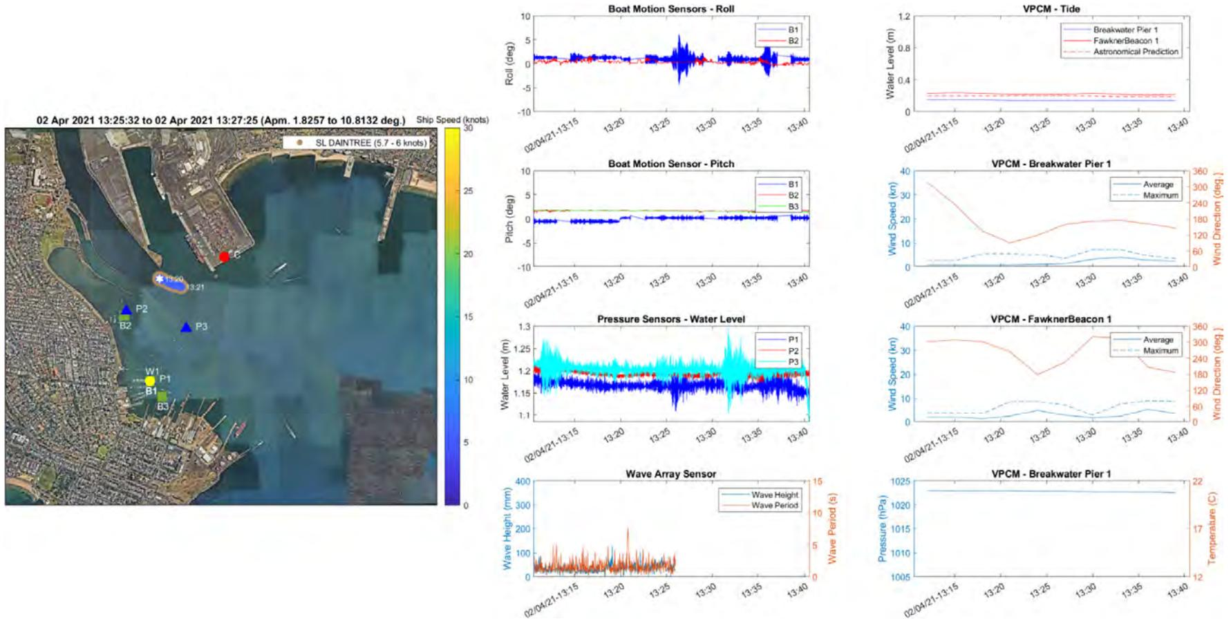
Figure 2.25 Summary diagnostic plot for example 1 of an event detection with only a Tug associated
