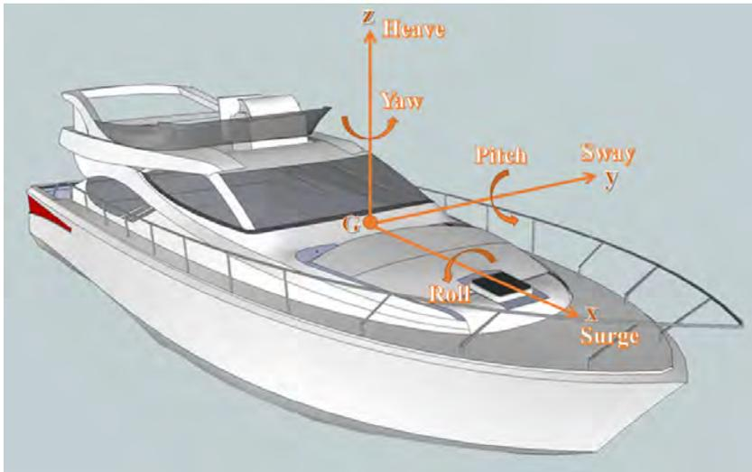
Figure 2.37 Schematic showing six degrees of freedom for boat motion
