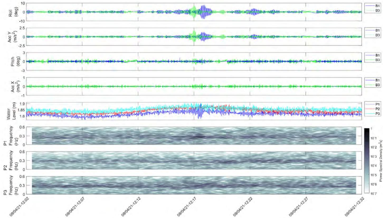
Figure 2.29 Spectrogram and diagnostic plot for example 2 of an event detection with only Tugs associated
