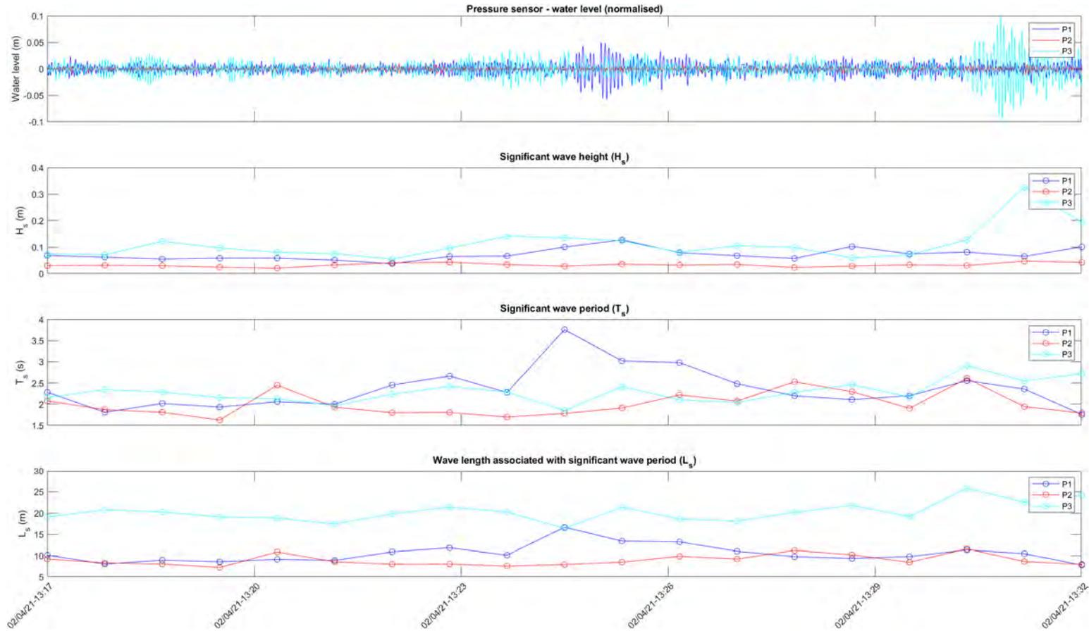
Figure 2.27 Wave characteristics determined from the pressure sensors for example 1 of an event detection with only a Tug associated
