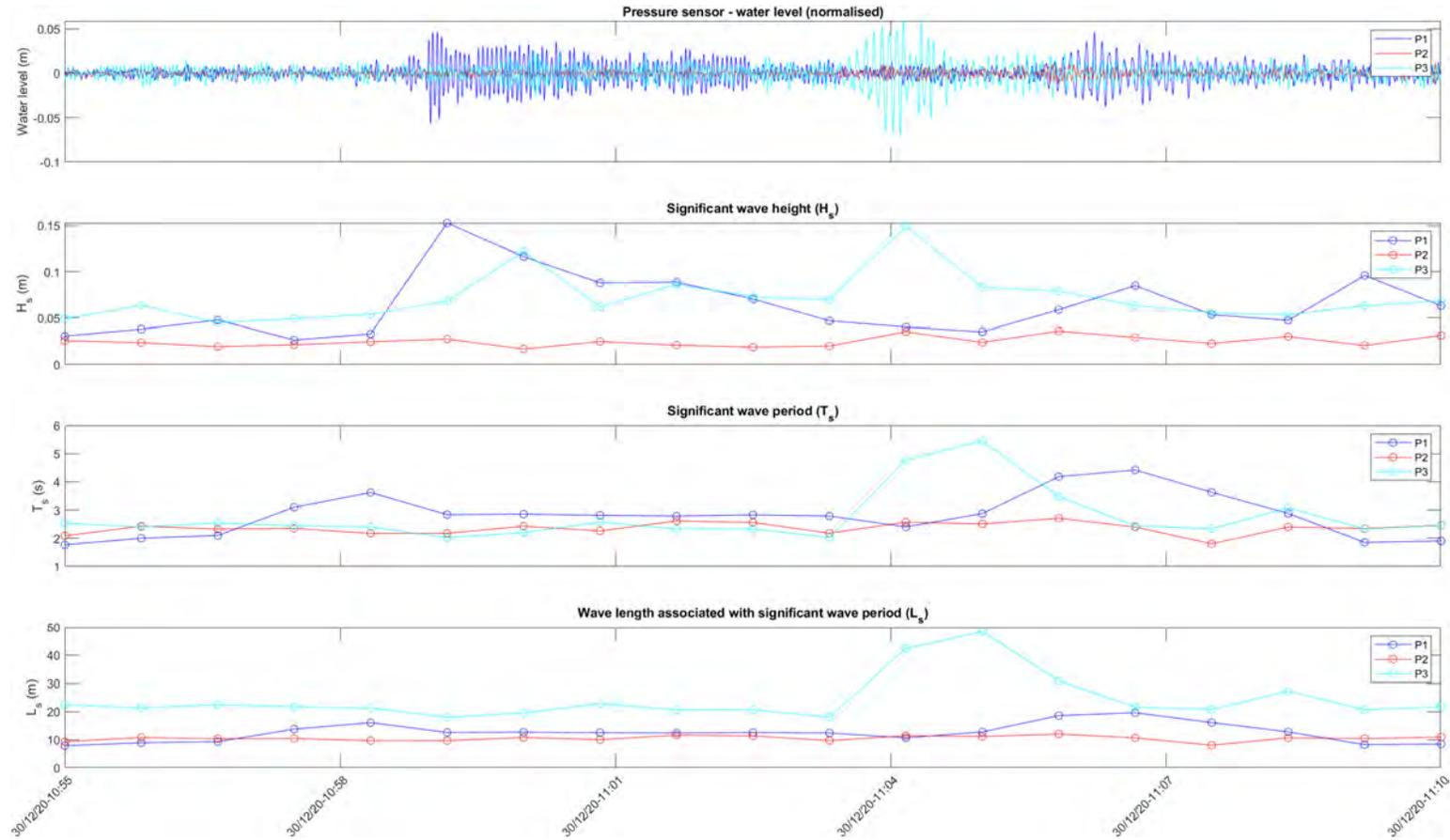
Figure 2.41 Wave characteristics determined from the pressure sensors for an example surge event (event No. 3 listed in Table 2.4)
