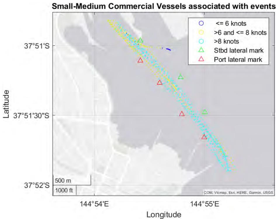
Figure 4.7 Vessel speed and location recorded in the AIS data during the collection period, for Small-Medium Commercial vessels (excluding SAR) associated with detected events
