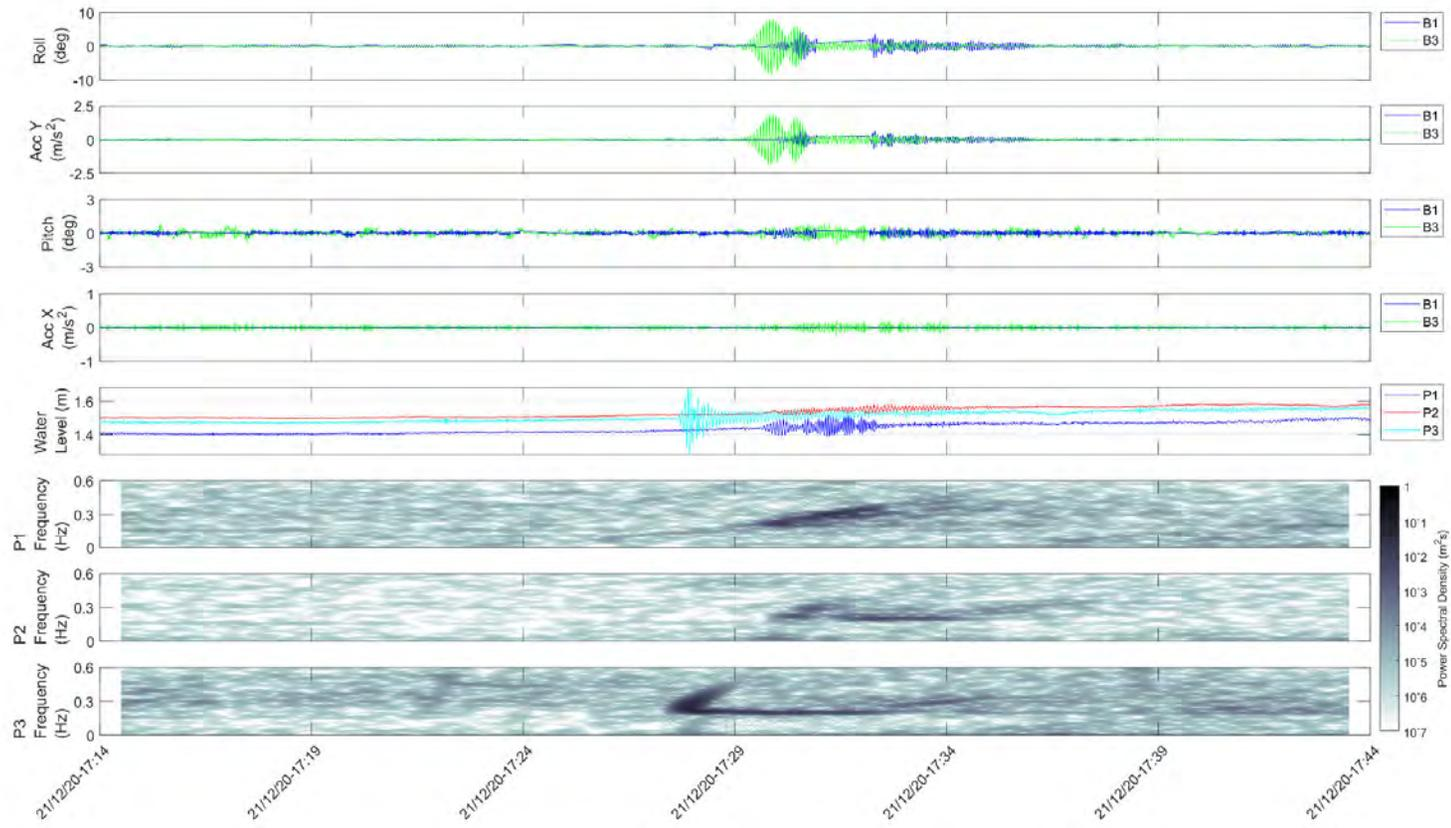
Figure 2.32 Spectrogram and diagnostic plot for example 1 event detection with a motorboat (Pleasure Craft) associated
