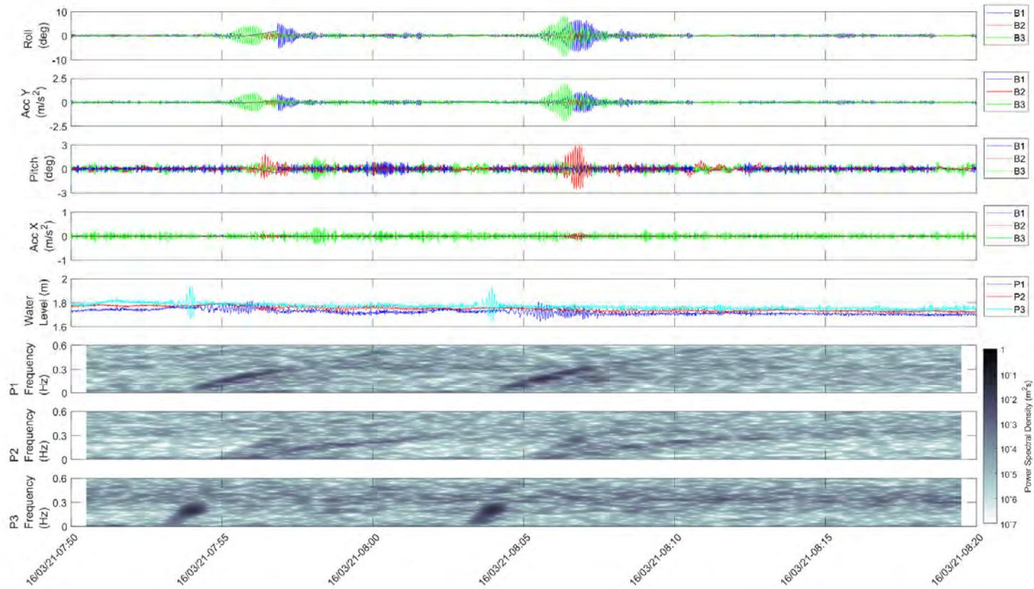
Figure 2.20 Spectrogram and diagnostic plot for an example event detection with only a Fast Ferry associated
