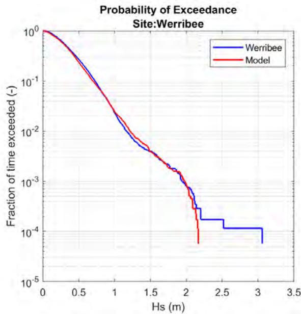
Figure 2.6 Probability of exceedance of model hindcast significant wave height and collocated Werribee Buoy observations
