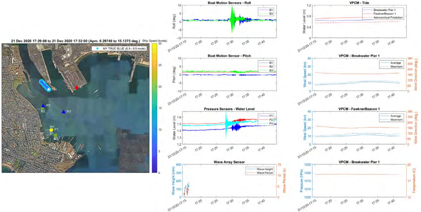
Figure 2.31 Summary diagnostic plot for example 1 event detection with a motorboat (Pleasure Craft) associated
