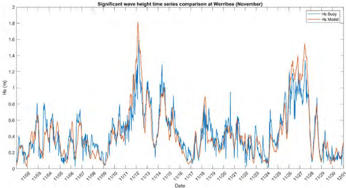
Figure 2.5 Wave timeseries from Werribee buoy (blue) and model hindcast (orange) for November 2021
