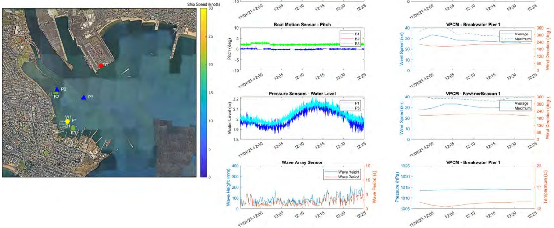
Figure 2.15 Summary diagnostic plot of marine traffic, metocean conditions and moored boat motions on 11 April 2021 from 11:55 to 12:25
