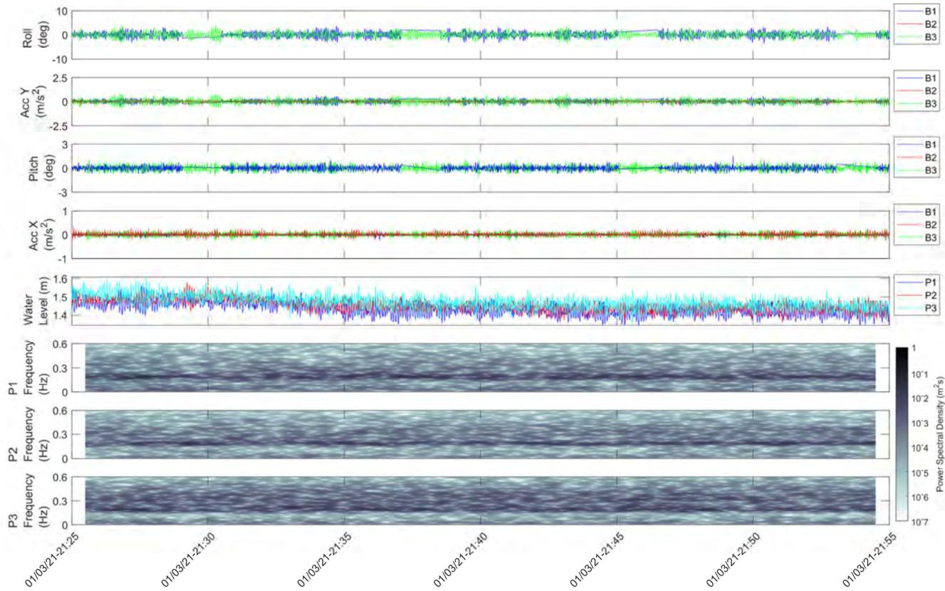
Figure 2.14 Spectrogram plot for metocean condition and boat motion accelerations on 1 March 2021 from 21:25 to 21:55
