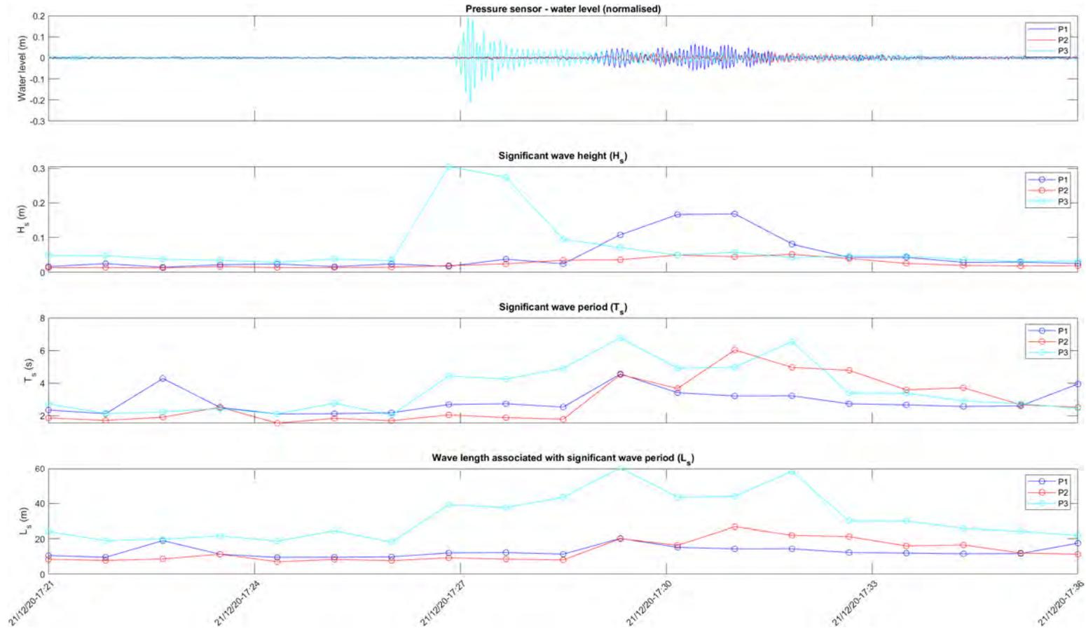
Figure 2.33 Wave characteristics determined from the pressure sensors for example 1 event detection with a motorboat (Pleasure Craft) associated
