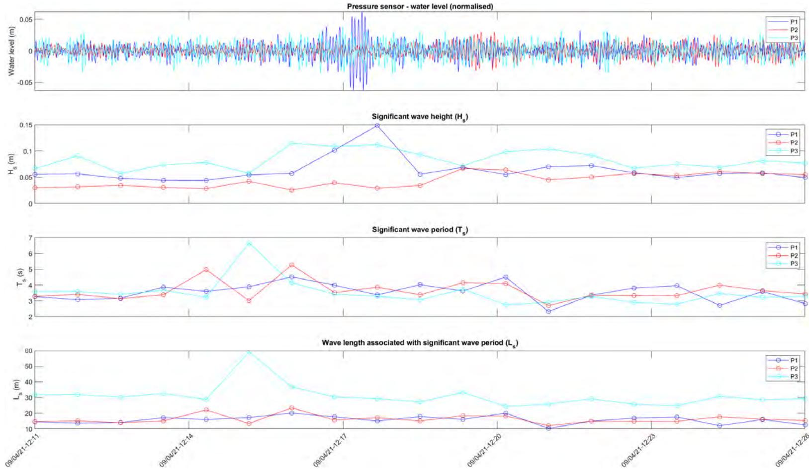
Figure 2.30 Wave characteristics determined from the pressure sensors for example 2 of an event detection with only a Tug associated
