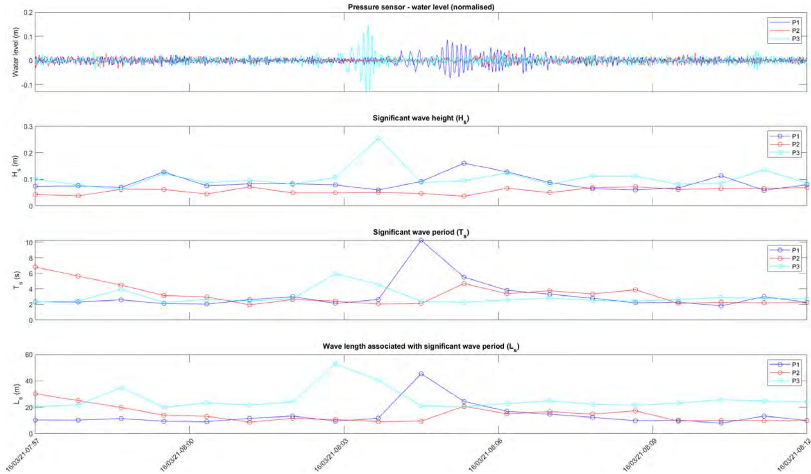
Figure 2.21 Wave characteristics determined from the pressure sensors for an example event detection with only a Fast Ferry associated
