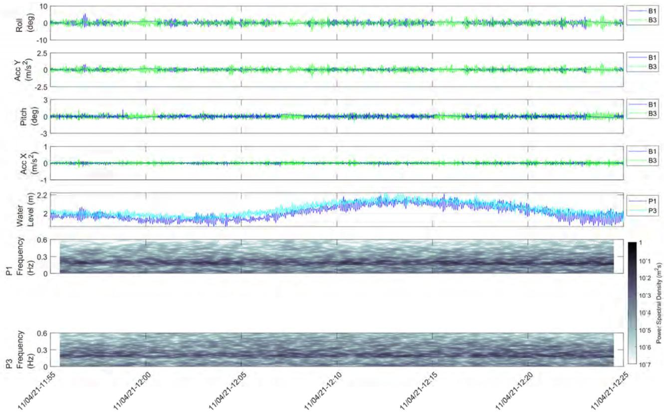
Figure 2.16 Spectrogram plot for metocean conditions and boat motion accelerations on 11 April 2021 from 11:55 to 12:25
