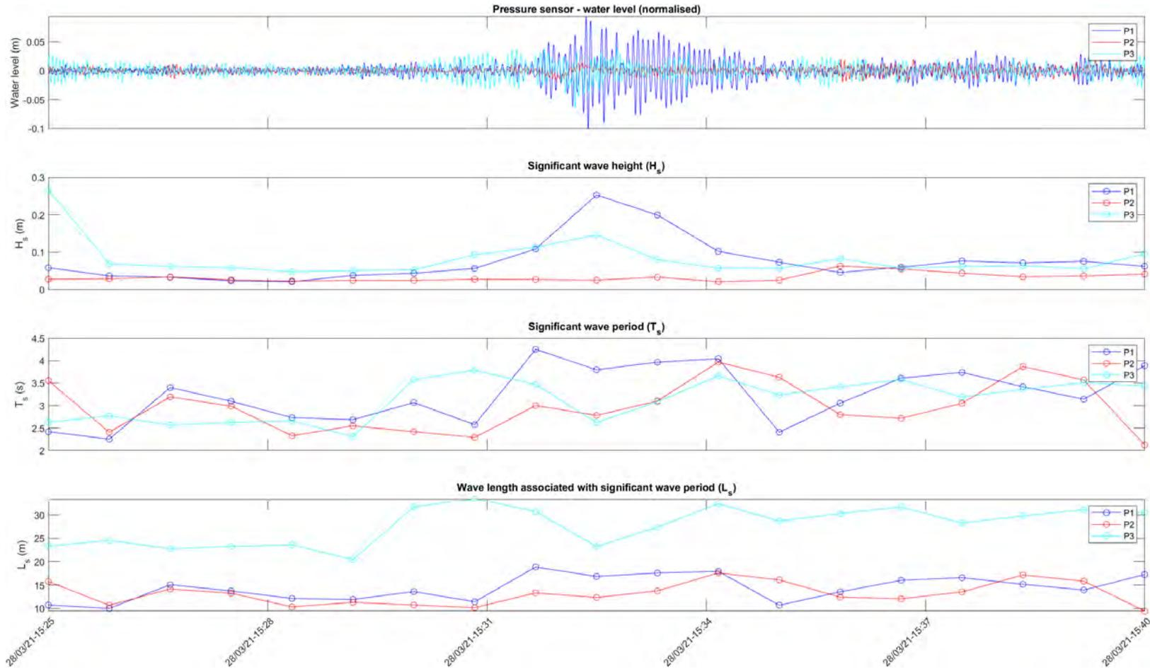
Figure 2.24 Wave characteristics determined from the pressure sensors for an example event detection with a passing Tanker vessel
