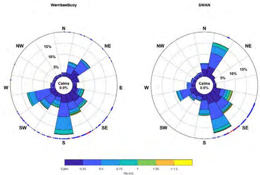
Figure 2.7 All-year Wave roses from buoy (left) and model hindcast (right).
