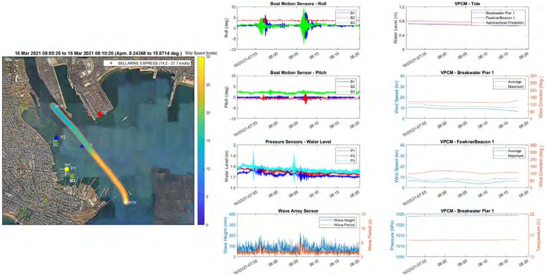
Figure 2.19 Summary diagnostic plot for an example event detection with only a Fast Ferry associated
