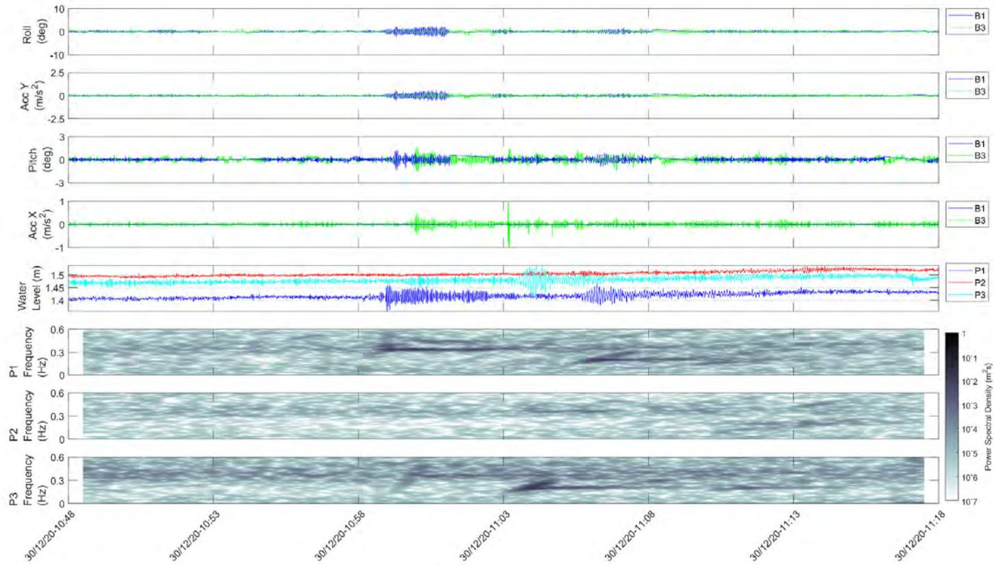
Figure 2.40 Spectrogram plot for an example surge event (event No. 3 listed in Table 2.4)
