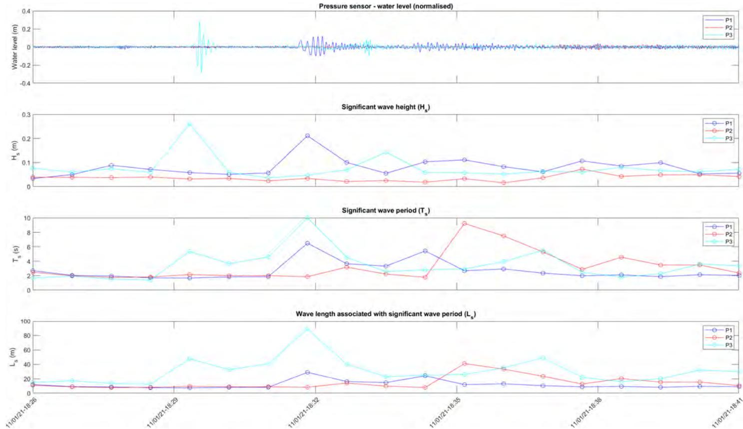
Figure 2.44 Wave characteristics determined from the pressure sensors for a reported surge event (event No. 7 listed Table 2.4 and further described as report No 4 in Table 2.5)
