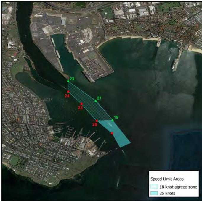
Figure 4.3 Diagram to show the 25-knot zone and voluntarily agreed 18-knot zone in the Williamstown channel
