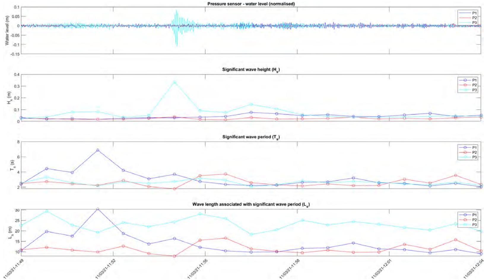
Figure 2.36 Wave characteristics determined from the pressure sensors for example 2 event detection with a motorboat (Pleasure Craft) associated
