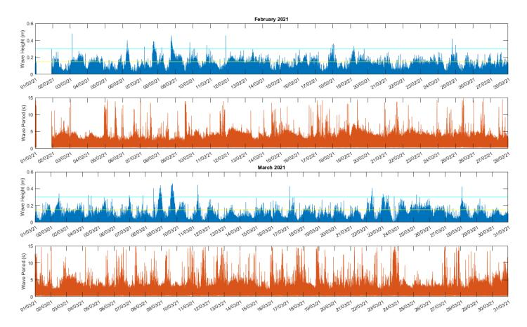
Figure 2.11 Measured wave height and period in February 2021 and March 2021 (the yellow and cyan lines represent the 0.15m and 0.30m wave heights recommended in AS 3962:2020 for "good" wave climate in marinas and boating facilities, refer to section 2.1.1 for further context)
