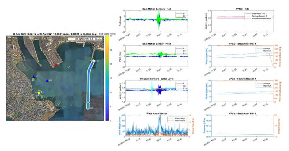
Figure 2.17 Summary diagnostic plot for a roll event of 19.6-degree maximum amplitude detected on 8 April 2021 at 10:33am
