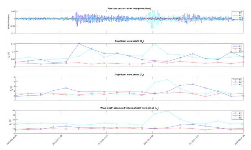
Figure 2.41 Wave characteristics determined from the pressure sensors for an example surge event (event No. 3 listed in Table 2.4)
