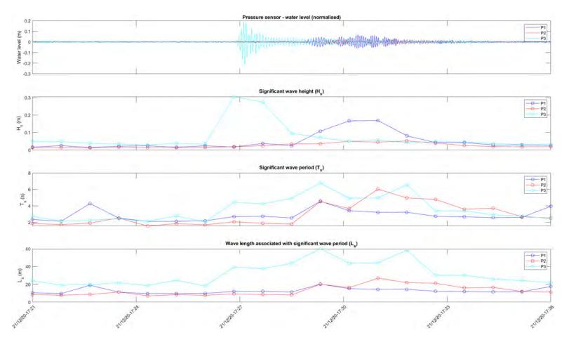
Figure 2.33 Wave characteristics determined from the pressure sensors for example 1 event detection with a motorboat (Pleasure Craft) associated
