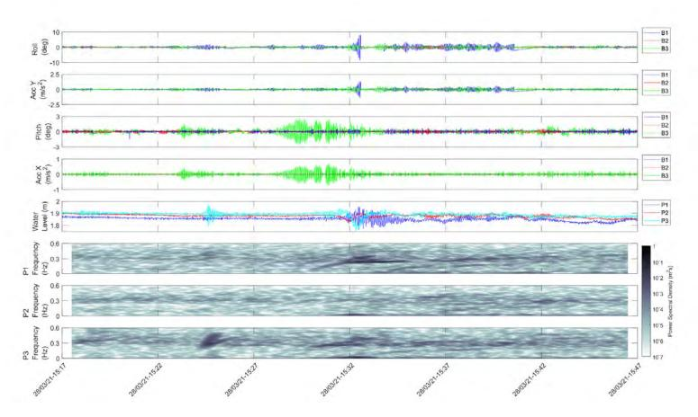
Figure 2.23 Spectrogram and diagnostic plot for an example event detection with a passing Tanker vessel
