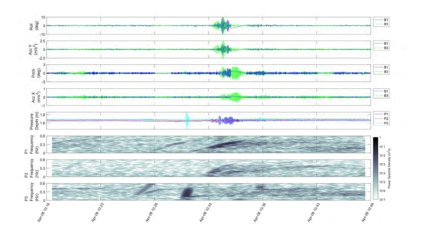
Figure 2.18 Spectrogram plot for metocean conditions and boat motion accelerations on 8 April 2021 from 10:18 to 10:48
