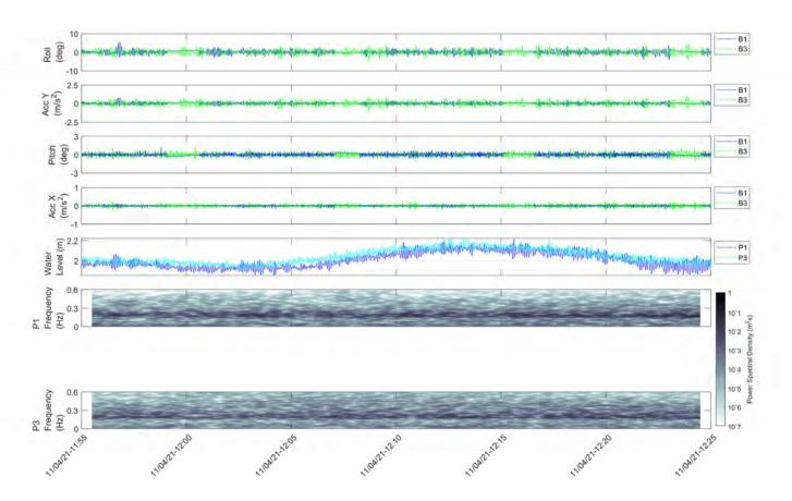
Figure 2.16 Spectrogram plot for metocean conditions and boat motion accelerations on 11 April 2021 from 11:55 to 12:25
