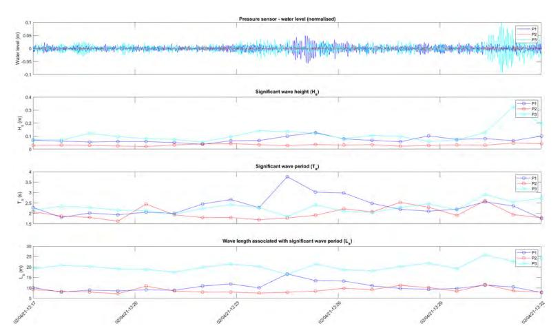
Figure 2.27 Wave characteristics determined from the pressure sensors for example 1 of an event detection with only a Tug associated
