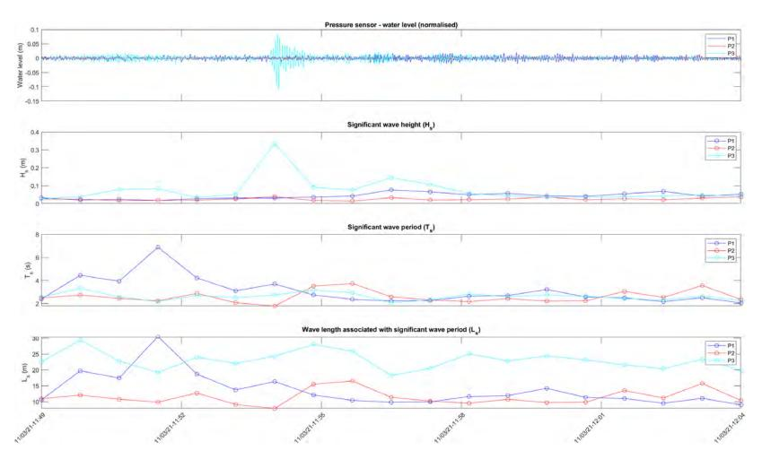
Figure 2.36 Wave characteristics determined from the pressure sensors for example 2 event detection with a motorboat (Pleasure Craft) associated
