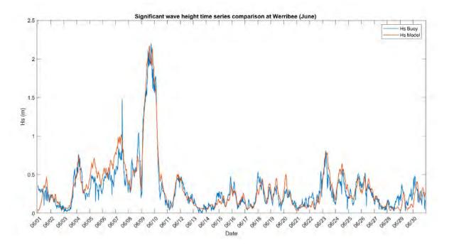
Figure 2.4 Wave timeseries from Werribee buoy (blue) and model hindcast (orange) for June 2021
