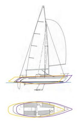
Figure 2.38 Diagrammatic representation of 'surge' motions of a vessel, back and forth along the bow-stern direction
