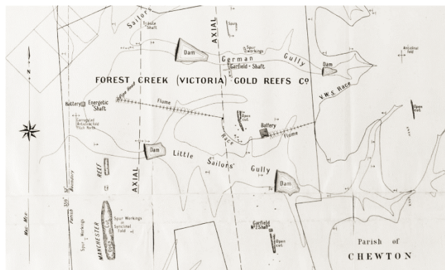
This plan of the Chewton Mines from 1902 shows the location of the Garfield and Energetic Shafts and the race and flume that took water from the Garfield Water Wheel to the former Manchester Company’s water wheel. Source: Mines Department, Earth Resources Regulation.
