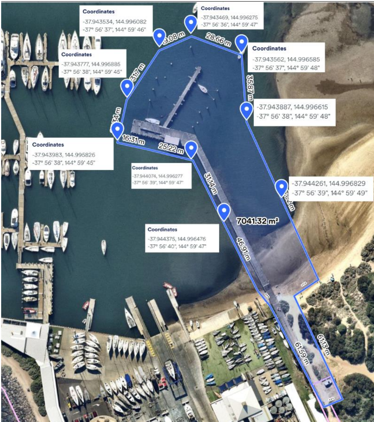
Figure 1 – Hampton Pier Demolition Works Exclusion Zone
